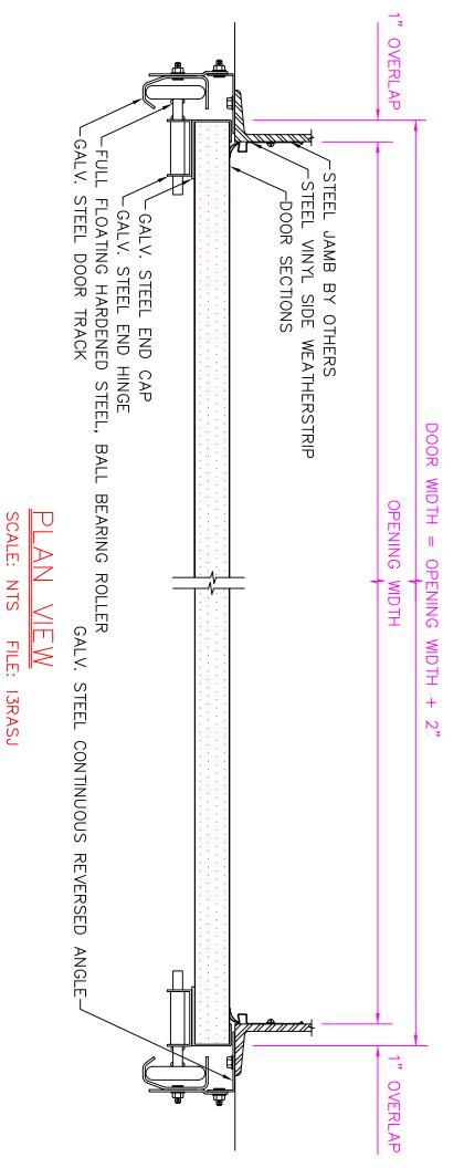
CONTINUOUS REVERSED ANGLE MOUNT - STEEL JAMB
